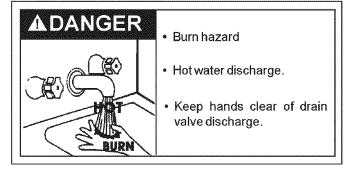
The water passing out of the drain valve may be extremely hot. To avoid being scalded, make sure all connections are tight and that the water flow is directed away from any person. 4. Remove the two screws securing the access panel, and remove panel.
